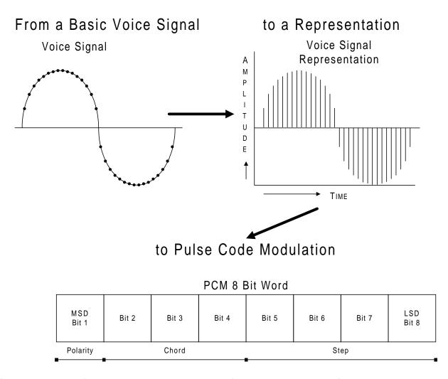
Standard PCM is 8000 samples/second, 8 bits/sample = 64k bit/sec
