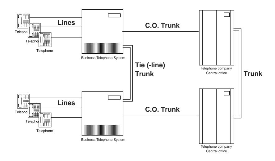
A *line* is a single circuit that connects a telephone to a switch
